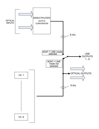
This mode enables the Scarlett OctoPre Dynamic to be used to connect an 8-channal ADAT format output (from a DAW, for example) to a set of analogue inputs, typically the channels of an analogue mixing console, to permit such a mixer to be used to mix down DAW tracks.
