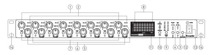
All operational controls and metering for all eight channels are on the front panel.
