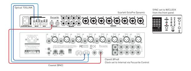
This example shows a similar setup to Example 2, but using a Focusrite Clarett 8PreX allows operation at a sample rate of 96 kHz ("SMUX-II" mode). Both units must be set to 96kHz; two optical cables are used, carrying four channels of audio each. The Clarett 8PreX is the sync master.
