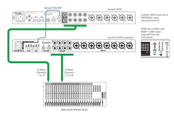
This example shows how to connect a greater number of DAW tracks to an analogue mixing desk for mixdown. The 10 analogue outputs of a Scarlett 18i20 interface are connected to desk Channels 1 to 10. Its **OPTICAL OUT** port is connected to an **ADAT IN** port of a Scarlett OctoPre Dynamic with ADAT > LINE mode selected. The OctoPre's **LINE OUTPUTS** are then connected to Channels 11 to 18 of the desk.
