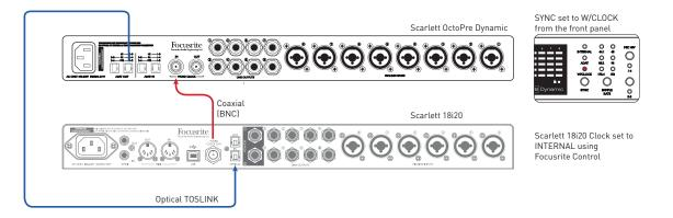
Here **ADAT OUT** on the Scarlett OctoPre Dynamic is connected to **OPTICAL IN** on a Scarlett 18i20 audio interface with a single optical cable. Both units are running at 44.1kHz sample rate. The OctoPre's **WORD CLOCK IN** input is connected to **WORD CLOCK OUT** on the Scarlett 18i20 with a BNC cable and the OctoPre's clock source is set to W/CLOCK. The 18i20's clock source is set to INTERNAL (via Focusrite Control), thus making it the sync master.
