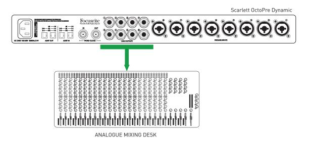
This setup uses the Scarlett OctoPre Dynamic's mic pre-amplifiers and compressors to provide a high quality "front end" for an analogue mixing desk. Use a pre-made loom to connect the OctoPre's **LINE OUTPUTS** socket to eight line inputs on the mixing desk; this will need eight ¼" TRS jacks on one end and eight connectors appropriate to the desk's line inputs on the other. If the desk's line inputs are unbalanced, a loom with TS jacks at the OctoPre end will be suitable.
