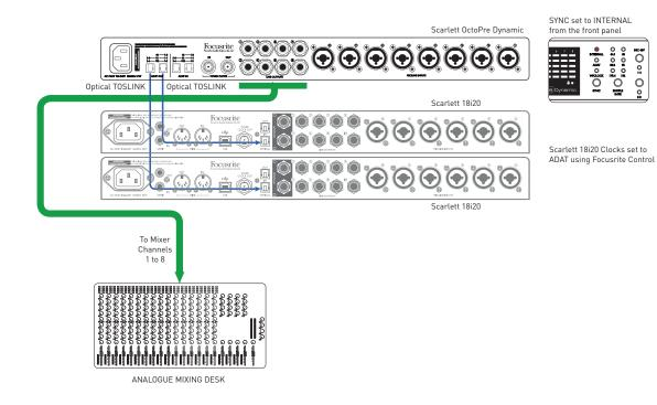
This example shows how the setup in Example 5 can be extended to add simultaneous digital recording, with or without secondary backup.
