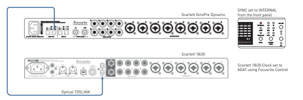
Here **ADAT OUT** on the Scarlett OctoPre Dynamic is connected to **OPTICAL IN** on a Scarlett 18i20 audio interface with a single optical cable. Both units are running at 44.1 kHz sample rate. The OctoPre's clock source is set to INTERNAL, and the 18i20 is synchronised to it because its clock source is set to ADAT (via Focusrite Control).
